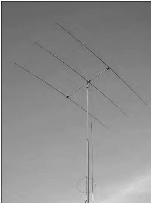
Figure 12-3: My three- element beam antenna.
